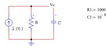
Define a voltage for the unknown node Vc(t). Current in the resistor can be calculated i.R(t)
